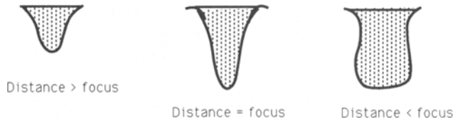
Fig. 22 Shapes of the cells resulting from engraving at the different distances between the last lens and the roll surface with regard to the focus of this lens
